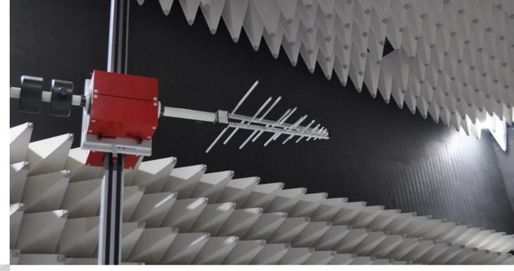
SAC-3 Transformed to a semi chamber with ground plane
