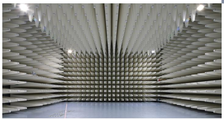
The innovative long-pyramid absorber technology achieves exceptional performance for emissions and immunity testing and offers highest homogeneity and impedance accuracy for the complete frequency range.
