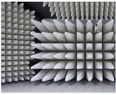
Due to the stable performance characteristics and its unique non-combustible attribute, a safe environment for people and EUT can be assured, which also leads to a constant, reproducible and long-lasting testing quality.
