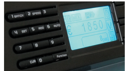
The numeric keyboard of V610 can be used for direct input batch counting values.
